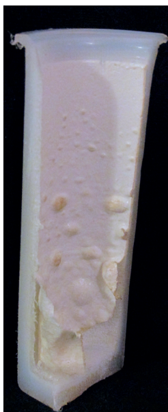
Figure 11. Damage to PFA microwave vessel after venting at high temperature.
