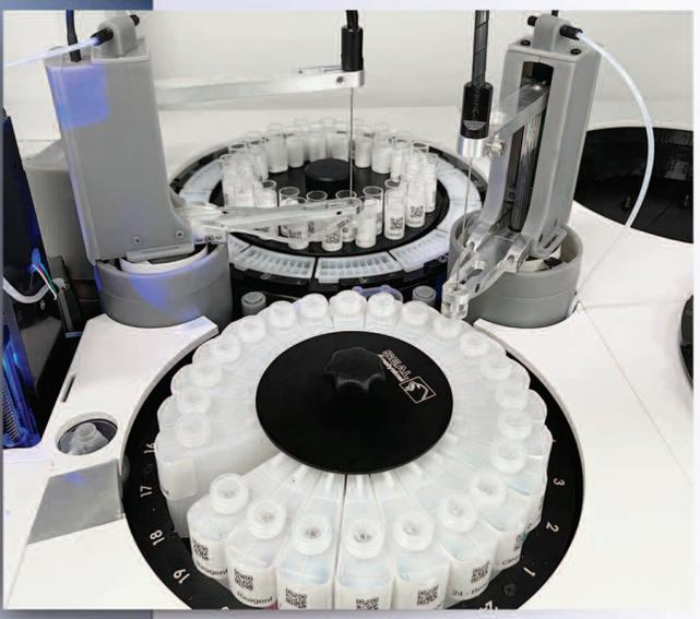
Colorimetric methods can be automated with a Discrete Analyzer. With no flow, baseline, peak shapes, pump tubes to monitor, hardware changes or shutdown procedures, your laboratory will achieve true "walk-away" analysis. After a run is finished the Discrete Analyzer even washes itself out and enters standby mode.
